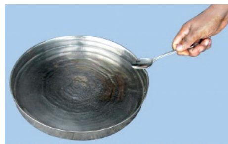
Fig. 7— Sound produced by a vibrating metal plate
